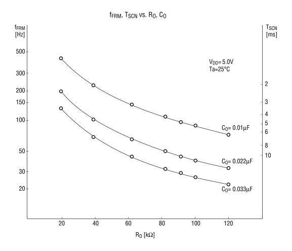
The frequency changes depending on supply voltages and temperatures. For  $V_{DD}$ , the frequency becomes about 5% higher at  $5\pm0.5V$  than at 5V. For temperature, the frequency becomes about 12% higher at  $T_{a}=40$ °C and becomes about 10% lower at  $T_{a}=85$ °C than at  $T_{a}=25$ °C. (The temperature characteristic of an external resistor and capacitor is not taken into consideration here.)
